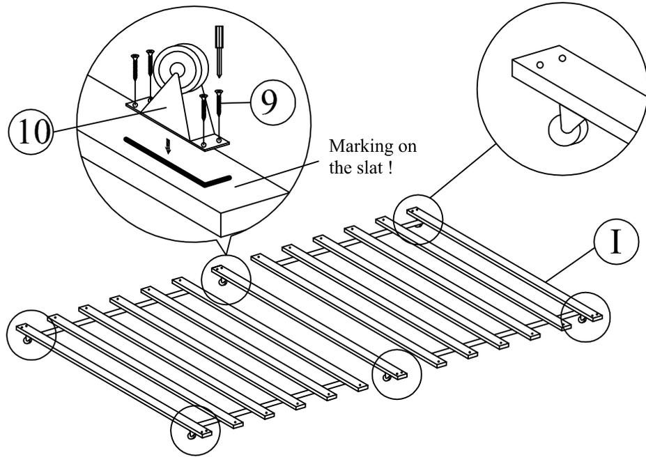
Step 6: Place the wooden blocks (J) at the corner of the trundle and fix the slat (I) to the side rail at (F) & (G) .
