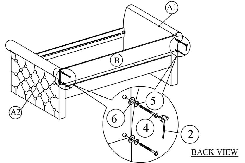
Step 3: Tighten the 4 Corner with Allen Key (1). Install the slats to side rail. Tighten the slats with CSK screw (3). The distance of the slats should be sufficient to obtain desirable bed stability.
